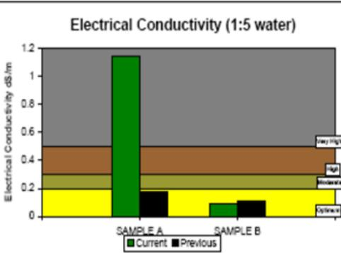
Electrical Conductivity (EC) is a convenient method for measuring soil salinity. The bar charts show June soil samples in Black and August samples in Green.
